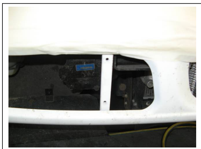
Figure 1: Drivers side mesh support. Remove from rear of bar using grinder or similar.
